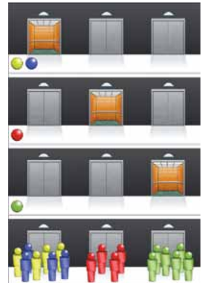
Destination based dispatching results in a low mix of destinations per car, requiring fewer stops and less time.
