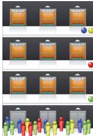
Traditional dispatching results in a high mix of destinations per car, requiring more stops and more time.
